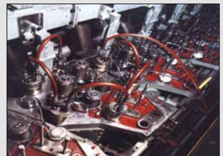
▲ Hydraulic nuts on a diesel engine.
