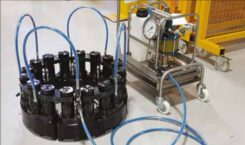
▲ Multi Stud Tensioning Set-Up.
